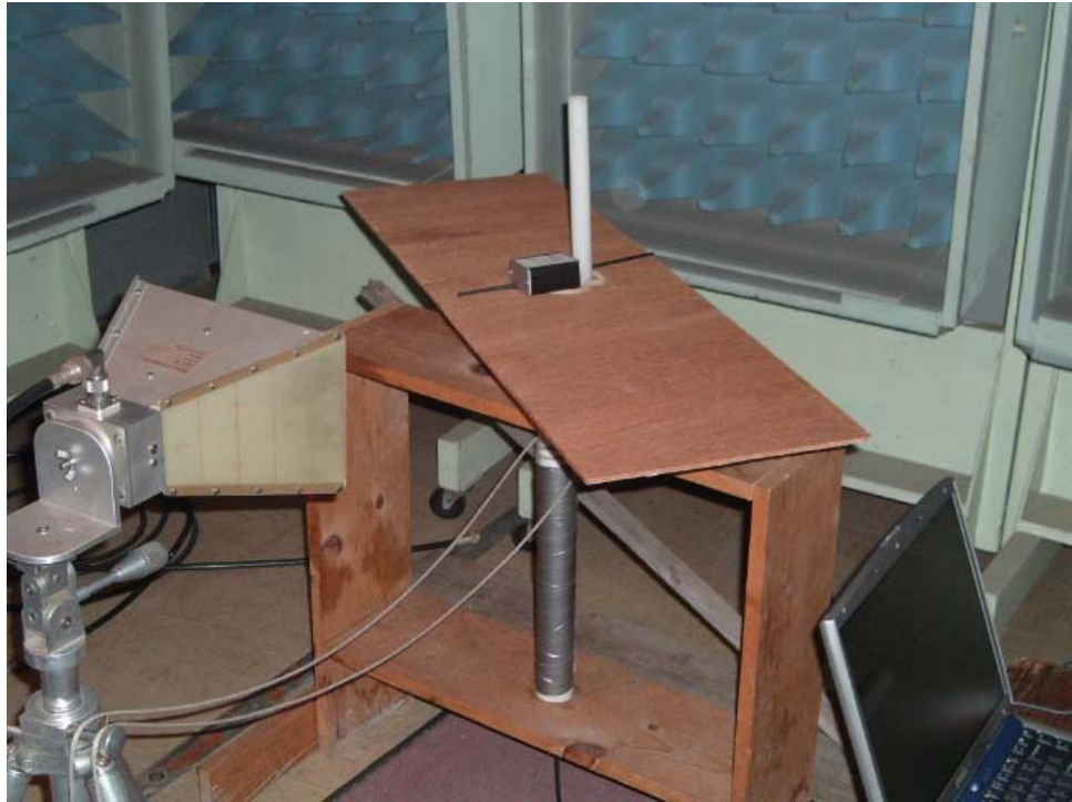
Pictorial 1 N9Y0085 Test Set-up Restricted Band Emissions
