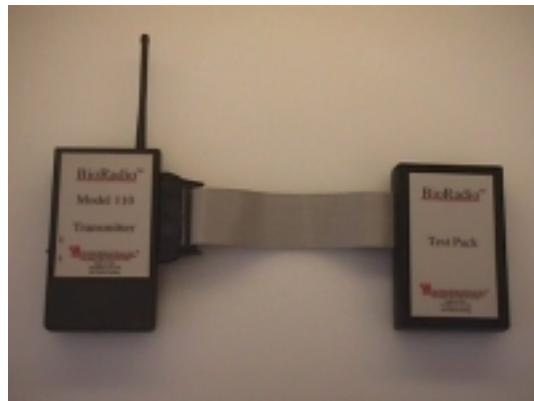
In order to determine the functionality of the system (e.g. to test for adequate transmission range within a building or for system troubleshooting) the end user can connect the transmitter to a Test Pack. The Test Pack continually inputs a known signal (low frequency sinusoid) to the transmitter, allowing a system functionality check independent of the application's signal sources.
