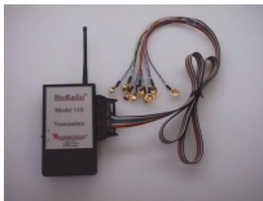
In this mode the transmitter is connected to the various source signals and continually transmits digitized data representing the acquired, processed signals. These input signals can number as few as one or as many as sixteen. Internal gain, filtering and digitization is applied to all the signals. Resulting data from all input signals is formatted into packets and transmitted to the receiver using a single RF frequency carrier.
