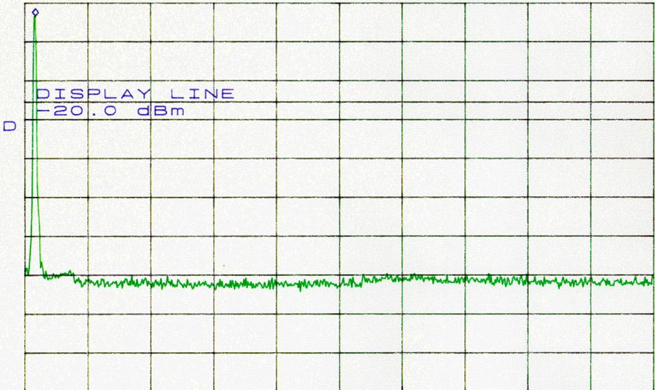
START 2.300GHzSTOP 10.000GHz\*RBW 100KHz\*VBW 300KHz\*SWP 2.0sec
