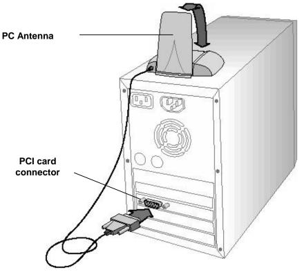
For best reception, locate the PC Antenna as high as possible and within four feet of your computer. Do not locate your PC Antenna where there is excessive vibration, heat, or moisture. The PC Antenna has an attached, 54-inch connector cable. Connect this cable to the SharePC PCI card connector.
