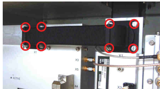
Fig. 7.49 WG SSPA, screws
