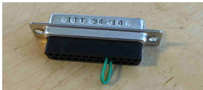
Fig. 7.1 25-pin D-SUB male connector with one wire
