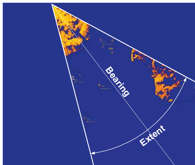
Fig. 5.13 Sector Bearing and Width
