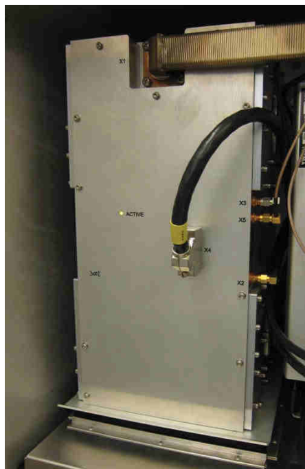
Fig. 3.2 200 watt SSPA with 4 x 50 watt PA modules. Note that a 50 watt SSPA is also available.
