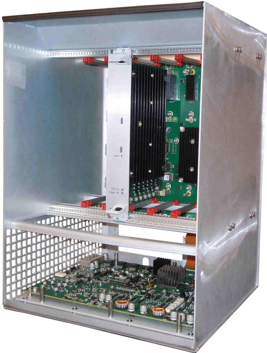
Fig. 4.16 Frame assy, shown with Ext. I/O and a CP4 board
