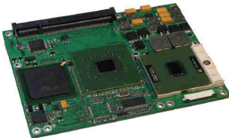
Fig. 4.20 PC Controller Board
