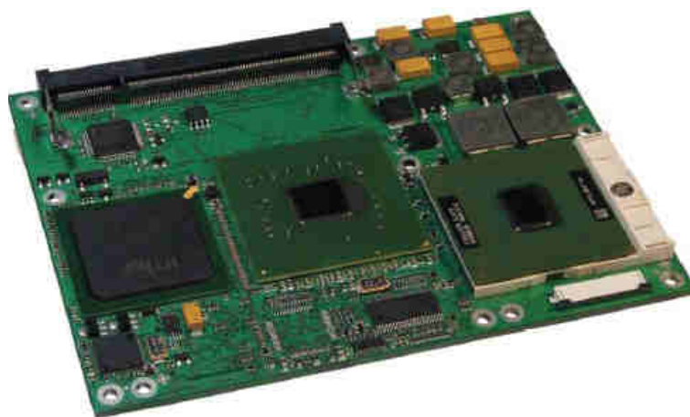
Fig. 4.21 PC Controller Board
