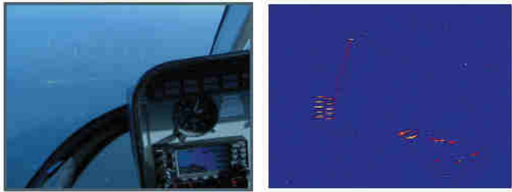
Fig. 3.14 Helicopter near wind turbine farm (left) and radar image of a helicopter near a wind turbine farm (right).
