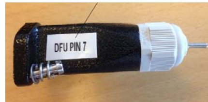
Fig. 6.2 Reset switch, X2 in DFU mode
