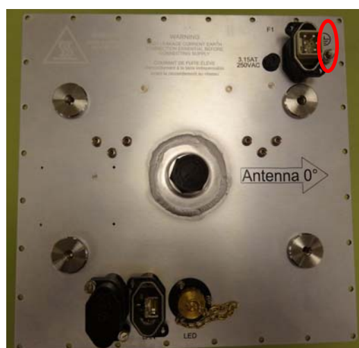
Fig. 4.2 Bottom plate, ground stud
