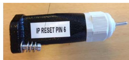
Fig. 6.1 Reset switch, X2 in IP reset mode
