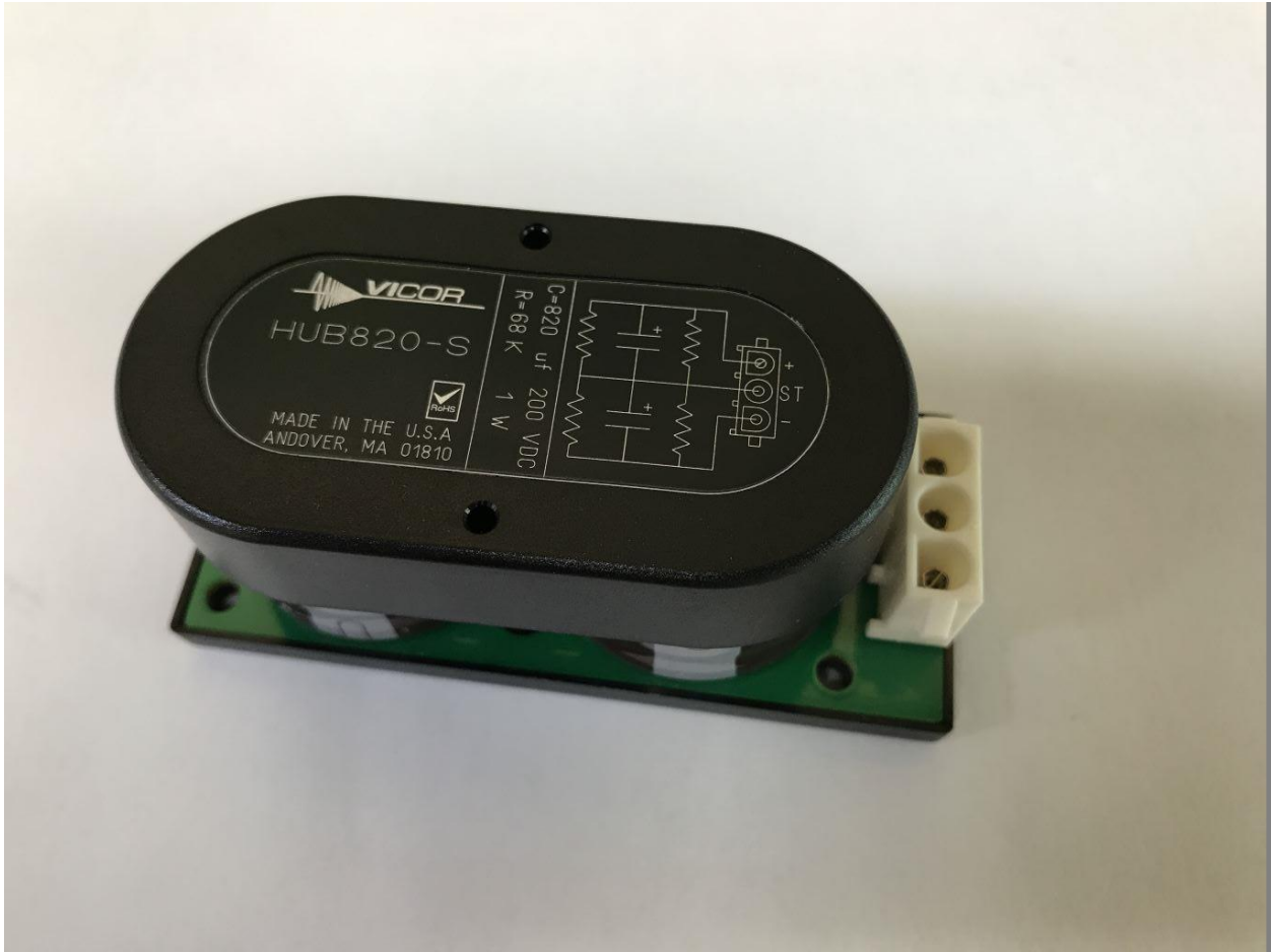
Power Supply Unit Module: Capacitor Bank Circuit Card Assembly
