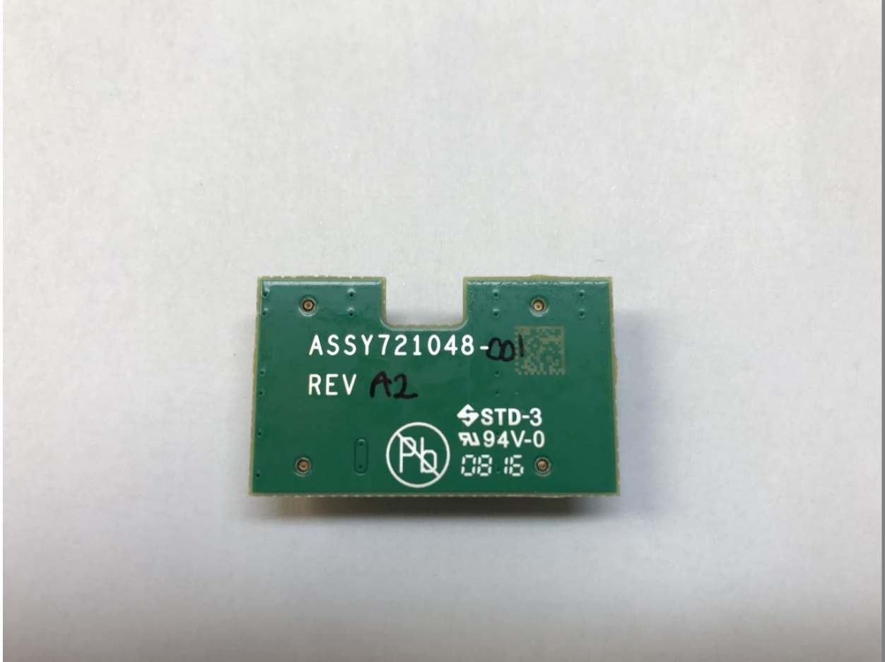
Transceiver Module: Bridge Circuit Card Assembly (Top)
