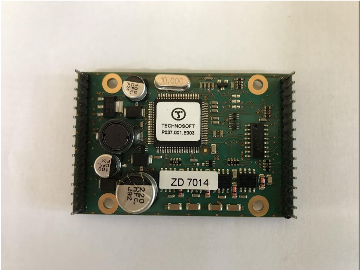
Motor Controller Module: Motor controller Circuit Card Assembly (Bottom)
