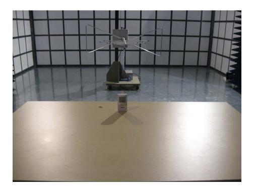
Radiation Emission Test Setup (Above 1GHz)
