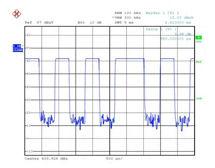
The graph shows the duration of 'on' signal. From marker 1 to marker 2, duration is 0.95 ms.
