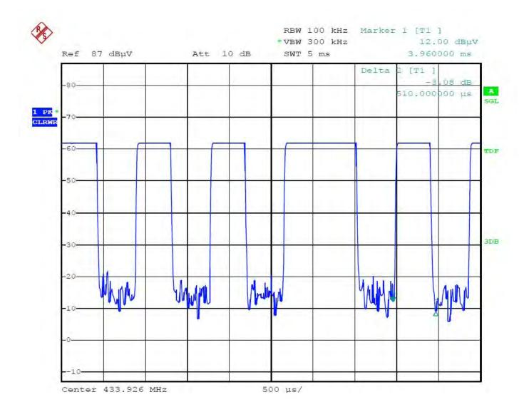
The graph shows the duration of 'on' signal. From marker 1 to marker 2, duration is 0.51 ms.
