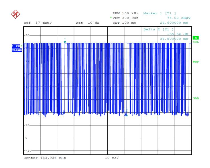
The graph shows the pattern of coding during the signal transmission. The duration of one cycle = 36.8 ms.
