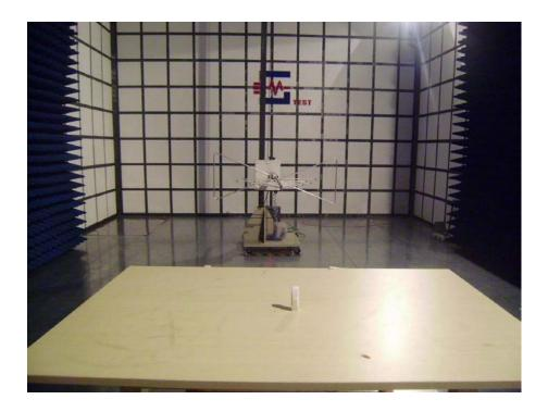
**Radiation Emission Test Setup (Above 1GHz)**
