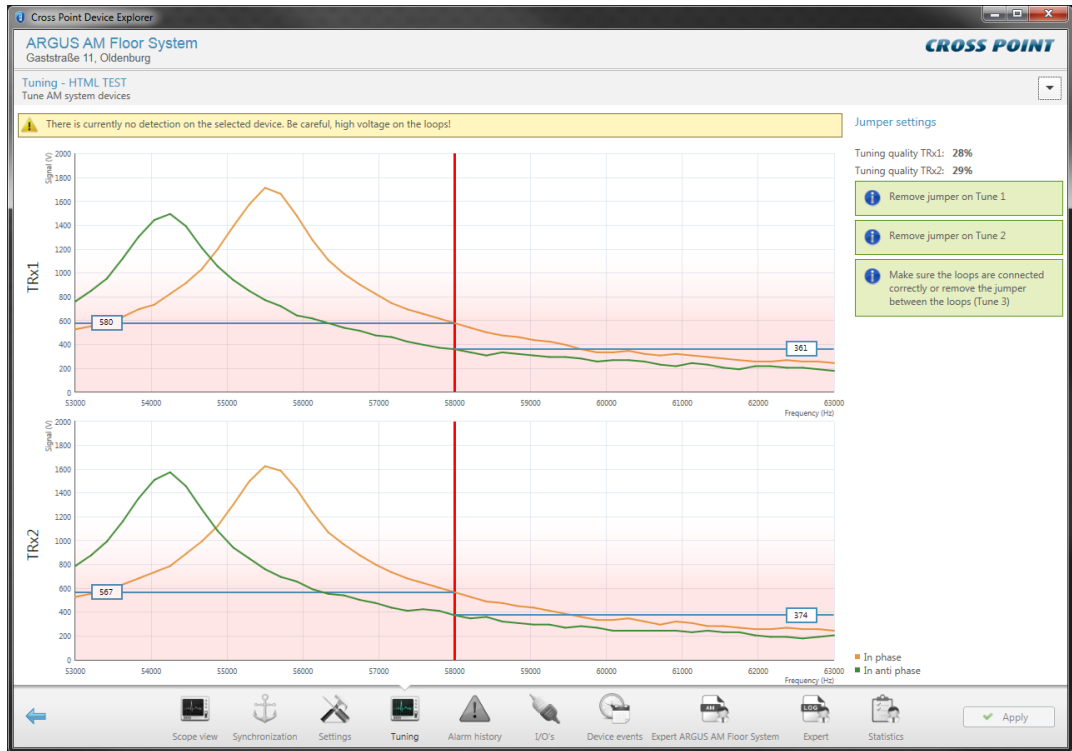
Figure 53: Visible tuning signals – tuning is not optimal yet
