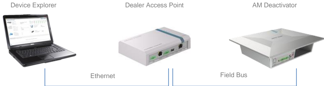
Figure 2: Field Bus connection
