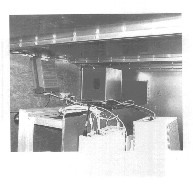
figure 4.2 conducted emission test setup
