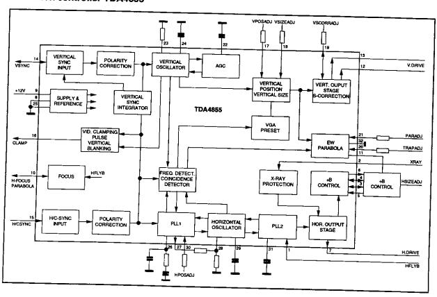
The TDA4855 contains the following blocks: Horizontal and vertical input The vertical sync signal enters at pin 14. It can have positive as well as negative polarity. The
