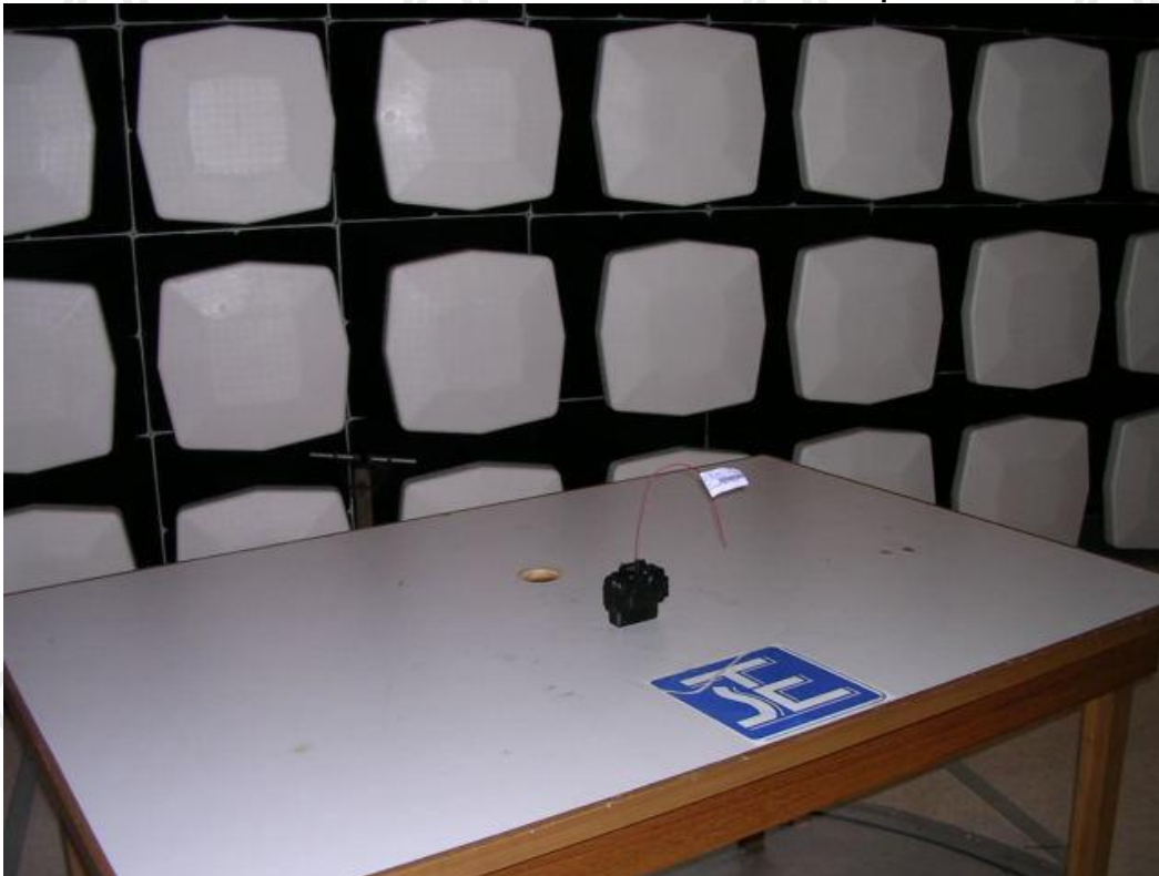
Measurement of Radiated Emission Test Set Up
