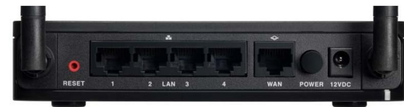
**RESET** Button—The **RESET** button has two functions:
