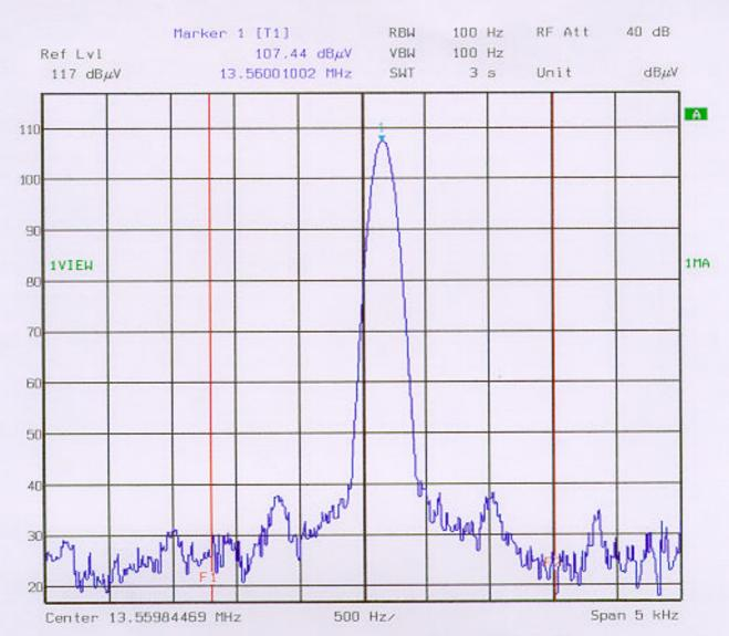
Comment A: Frequency error for Hasbro. Frequency Tolerance 0.01% 10.35Volts at -20degs.
