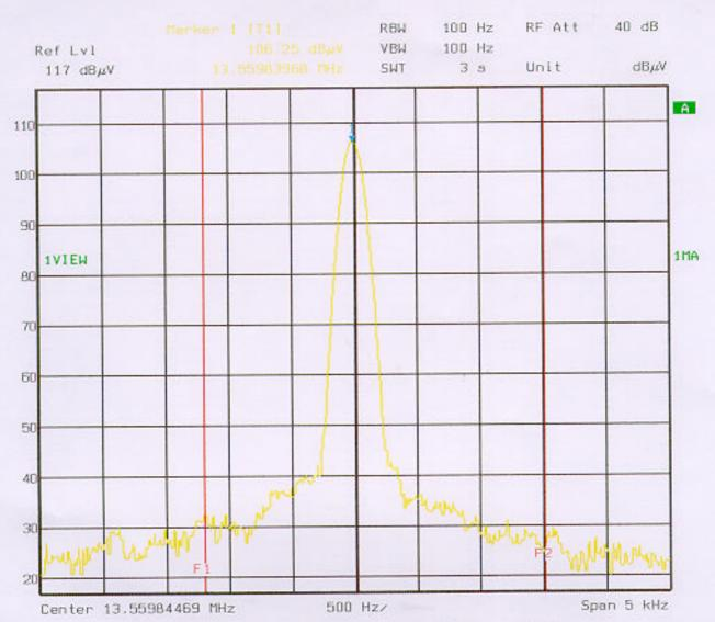
Comment A: Frequency error for Hasbro. Frequency Tolerance 0.81%
