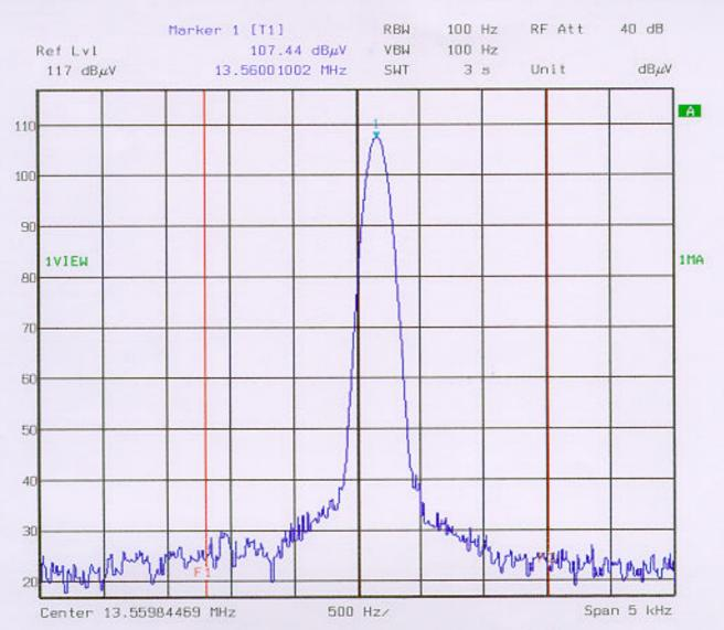
Comment A: Frequency error for Hasbro. Frequency Tolerance 0.01% 9.0Volts at -20degs.
