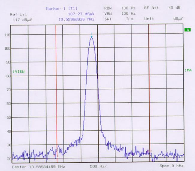
Comment A: Frequency error for Hasbro. Frequency Tolerance  $0.01 \times$
