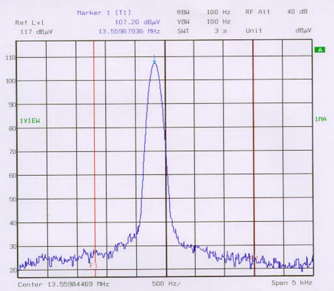
Comment A: Frequency error for Hasbro. Frequency Tolerance 0.01%
