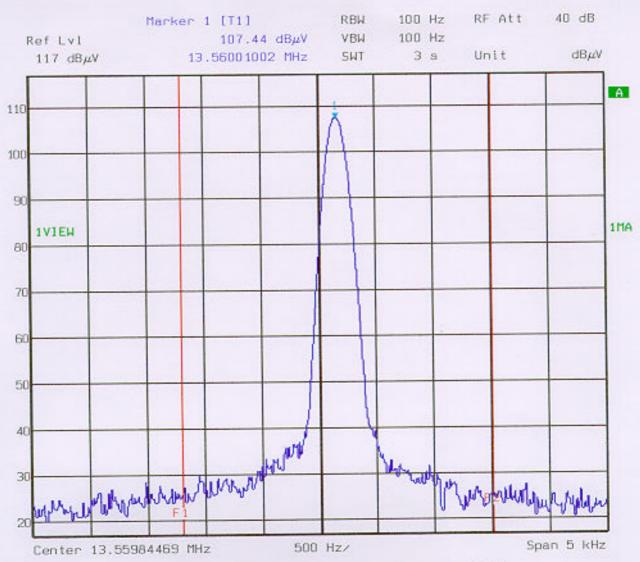
Comment A: Frequency error for Hasbro. Frequency Tolerance 0.01% 7.65Volts at -20degs.
