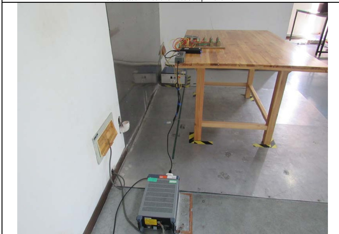
Conducted Emissions Test Setup Side View
