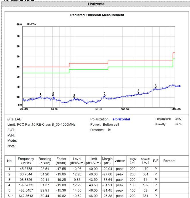
Note:1).Level ( $dB\mu V/m$ )= Reading ( $dB\mu V$ )+ Factor (dB/m)
