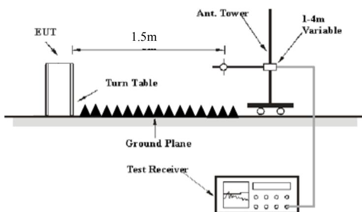
The radiated emission tests were performed in the 3 meters chamber test site, using the setup accordance with the ANSI C63.10-2013. The specification used was FCC 15.209, FCC 15.407 limits.
