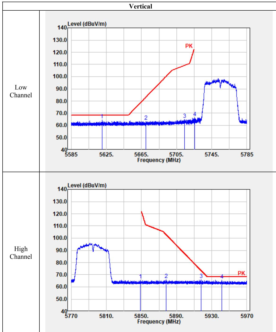
**Listed with the worst harmonic margin test plots (802.11ac vht80 5775 MHz)**
