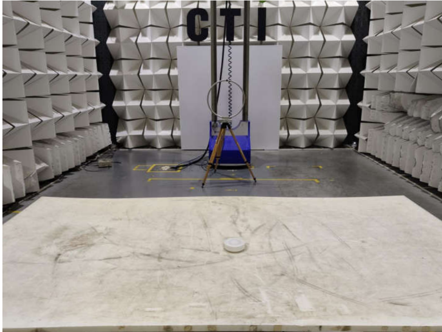
Radiated spurious emission Test Setup-1(Below 30MHz)
