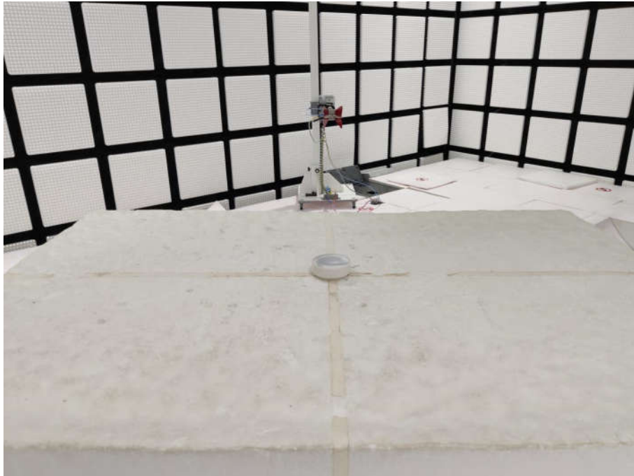
Radiated spurious emission Test Setup-3(Above 1GHz)
