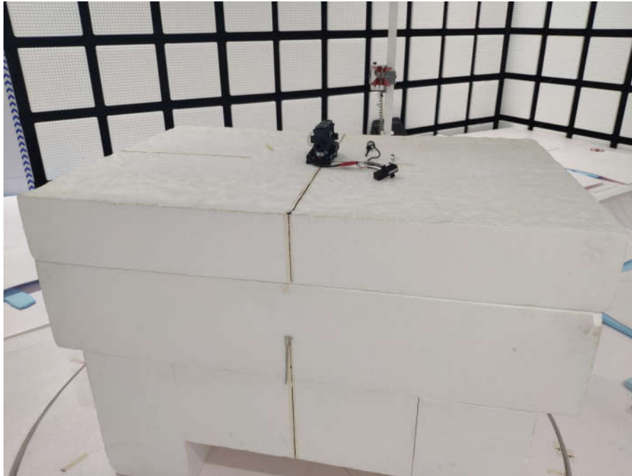
Radiated spurious emission Test Setup-2(Above 1GHz)
