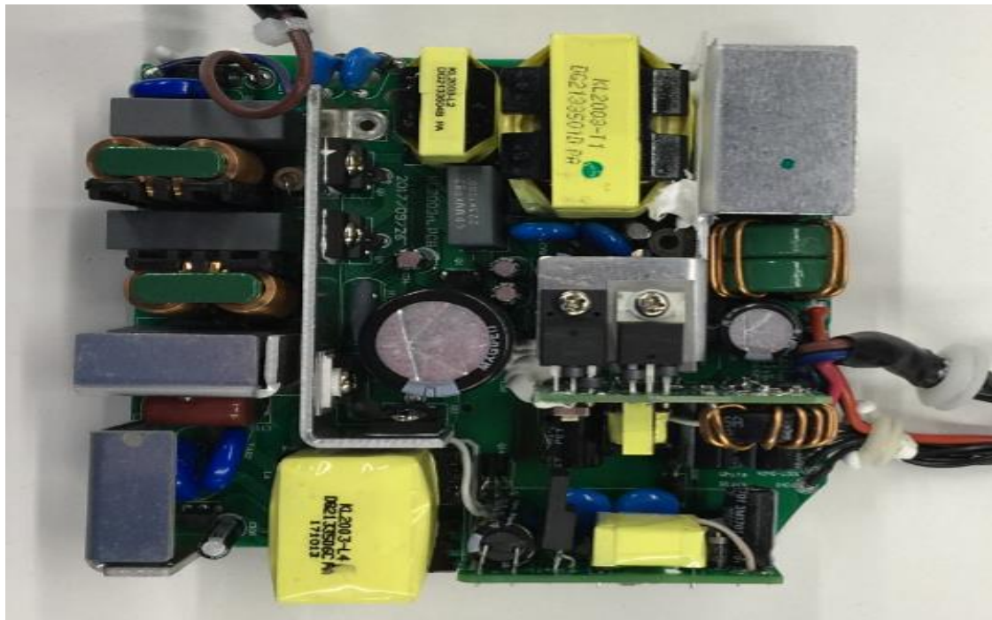
218W Power board using in K-5401-PA.
