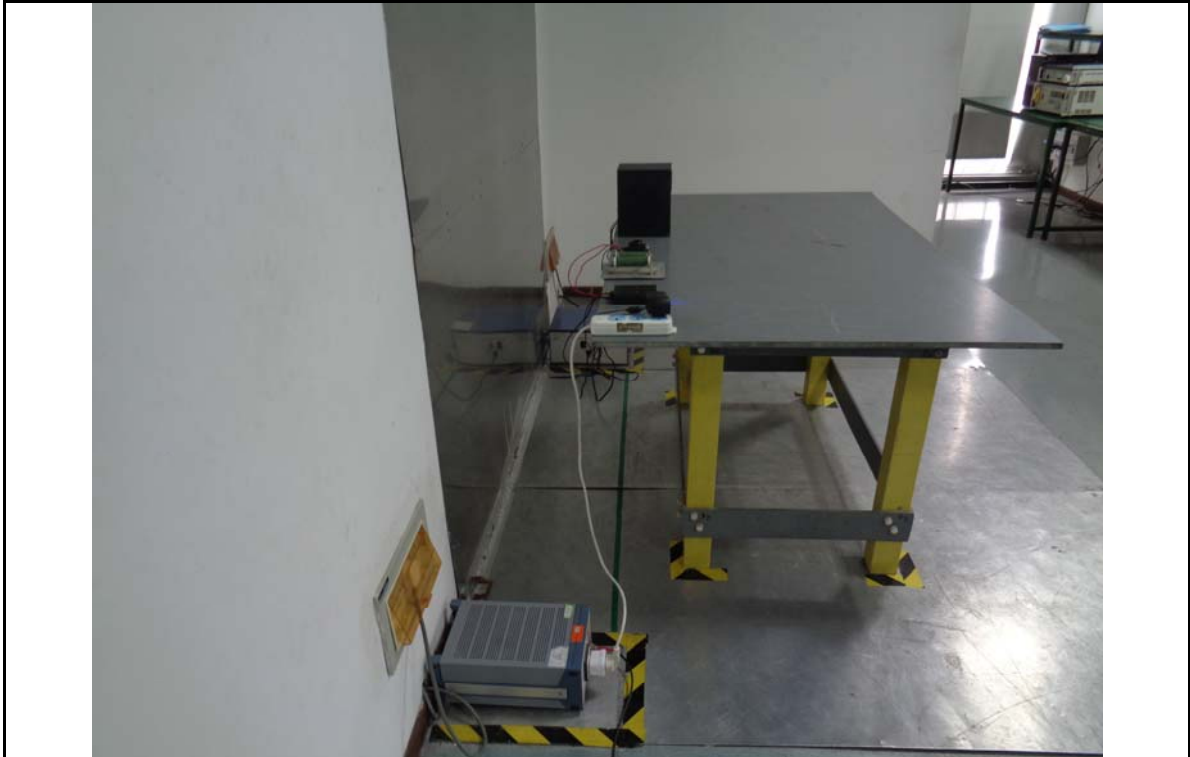
Conducted Emissions Test Setup – Side View
