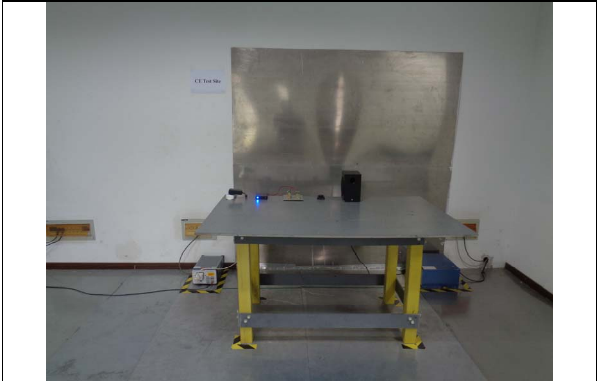
Conducted Emissions Test Setup – Front View
