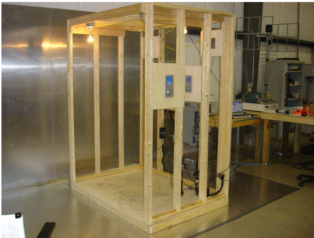
Figure 6. Overall Power Line Conducted Emissions Setup.
