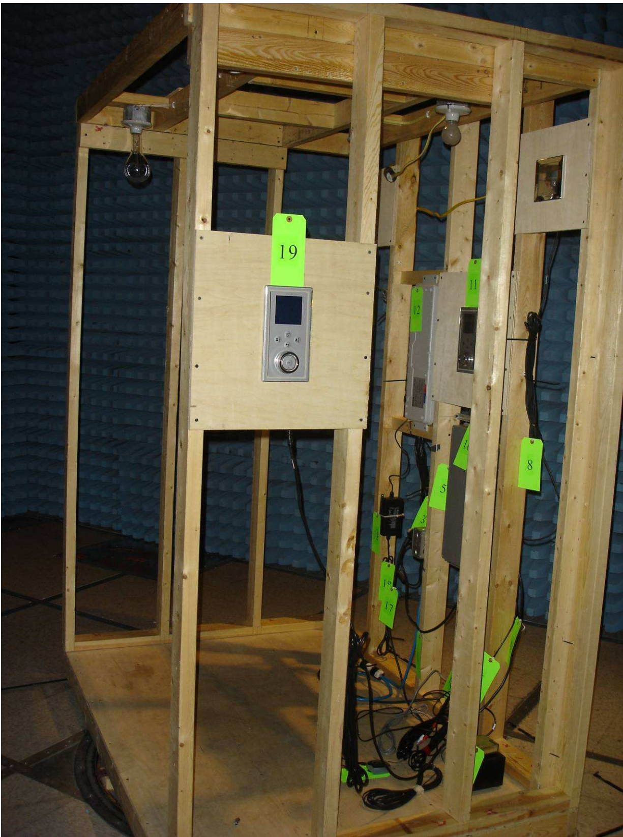
Figure 2. Side View of Peripheral (Digital Interface) Associated with Media Module (EUT) (Radiated Emissions)
