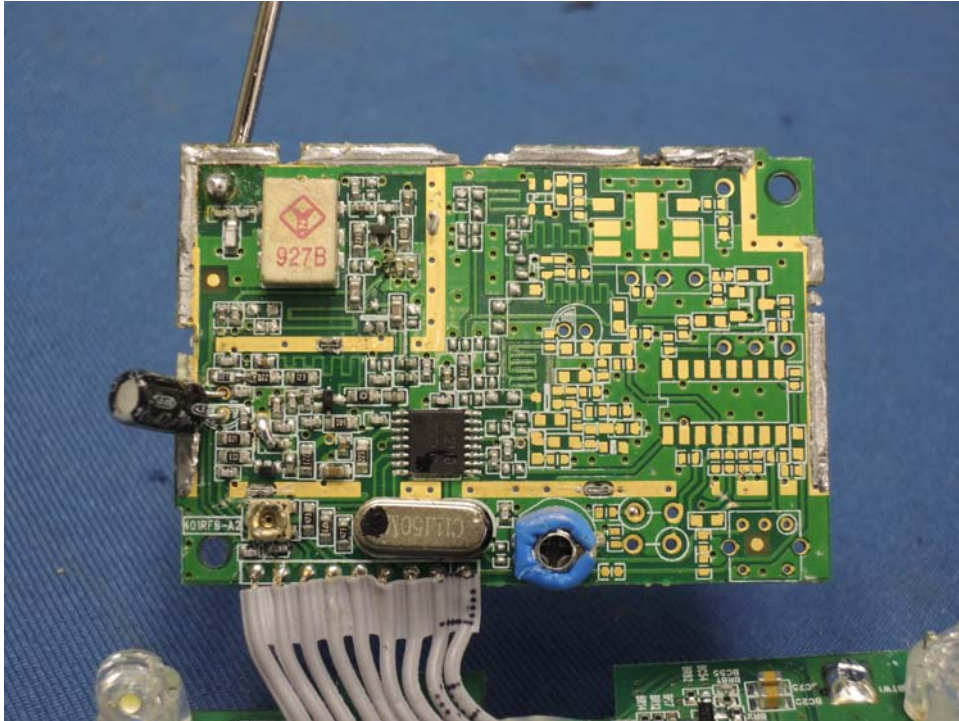
Baby Unit Oscillator PCB comp side (View 2)
