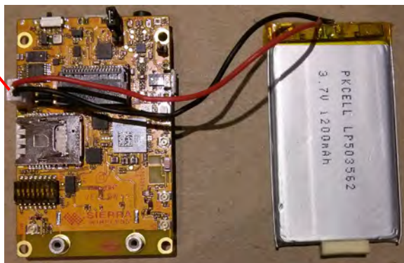
Figure 3-5: mangOH Yellow With Rechargeable Battery Connected
