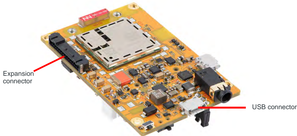
Figure 3-4: Power Supply Connectors
