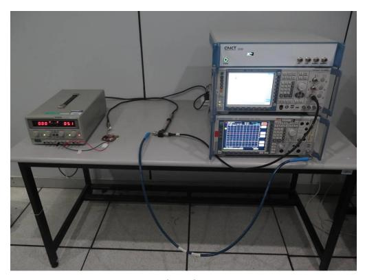
Pic.1 Conducted test set-up
