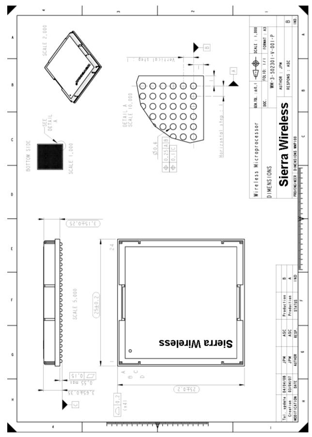
Figure 2. Mechanical Drawing of WMP100 (Top View)
