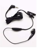
For maximum sound quality, be sure to push the mono headset connector all the way into the phone so that no rings on the connector are showing.
