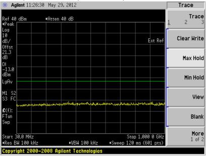
Plot 6.4.23) Out of Band Emissions at Antenna Terminals
