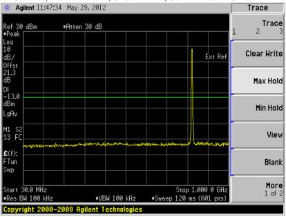
Plot 6.4.38) Out of Band Emissions at Antenna Terminals
