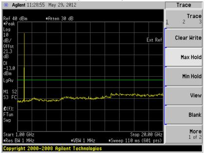
Plot 6.4.25) Out of Band Emissions at Antenna Terminals
