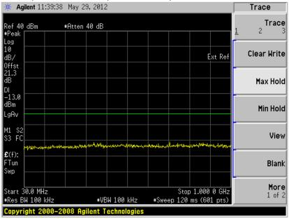
Plot 6.4.32) Out of Band Emissions at Antenna Terminals
