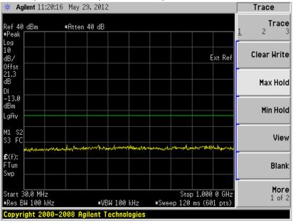
Plot 6.4.20) Out of Band Emissions at Antenna Terminals
