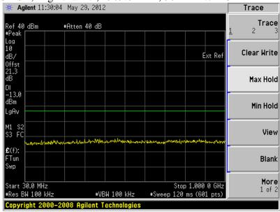
Plot 6.4.26) Out of Band Emissions at Antenna Terminals
