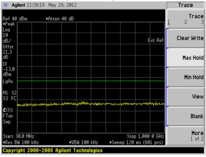
Plot 6.4.29) Out of Band Emissions at Antenna Terminals
