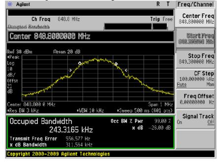
5.3.4) 8-PSK Occupied Bandwidth, Cellular Low channel, 824.2 MHz, 99% BW
