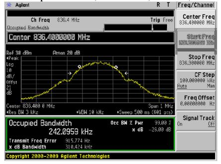
5.3.6) 8-PSK Occupied Bandwidth, High channel, 848.8 MHz, 99% bandwidth
