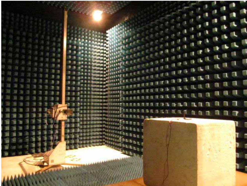
Description: Spurious Emission Above 1G Test Setup
