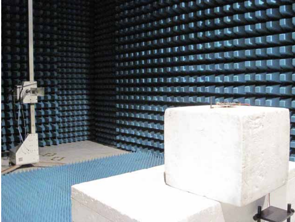
Description: Spurious Emission Above 1G Test Setup
