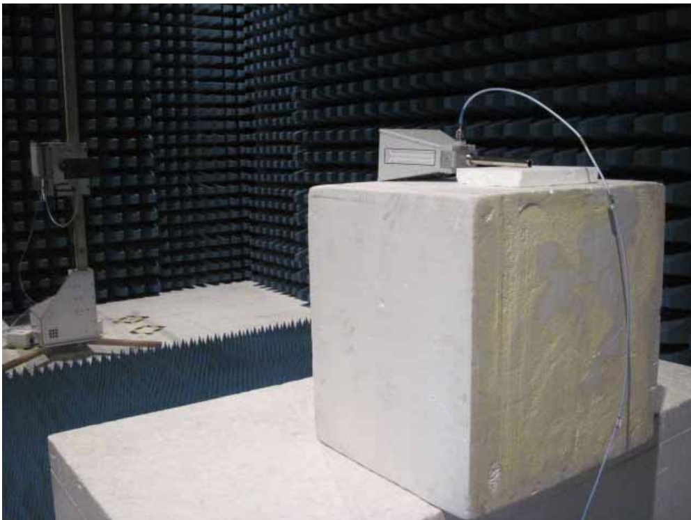
Description: Substitution Antenna for Spurious Emission Above 1G Test
