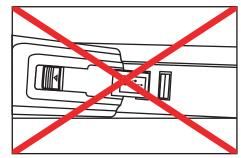
Figure 3-4: Wrong way to insert the USB modem
