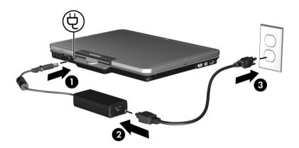
When the computer receives AC power, the battery begins to charge and the battery light (on the front of the computer) turns on. When the battery is fully charged, the battery light turns off.
