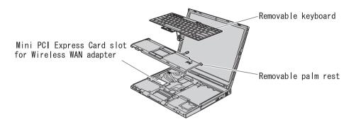
**Attention:** The ThinkPad T60 Series computer contains an authentication mechanism If you install an unauthorized wireless WAN Mini PCI Express Card that is not approved for use in the ThinkPad T60 Series computer, the computer will not start, but only displays an error message and emits beeps.
