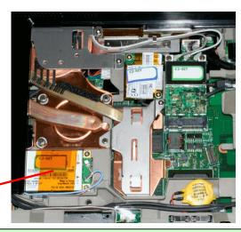
The certification label is stuck on the topside of the applying transmitter device, the FCC ID is visible when the keyboard assembly is removed.
