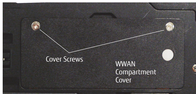
Figure 1. Removing WWAN cover
