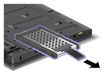
6. Detach the side spacer rails from the hard disk drive.
