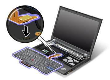
2. Insert the keyboard. Make sure that the rear edges of the keyboard are under the frame as shown by the arrows.
