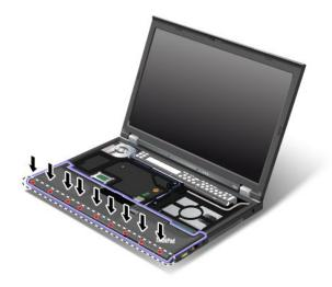
3. Attach the flip-lock ZIF connector 1, then push the palm rest cable 2.
