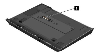
1 The docking connector is used for attaching the ThinkPad computer to the ThinkPad Battery 19+.
