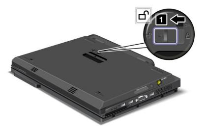
2. Release the eject lever 2 and pull up the ThinkPad Battery 19+.
