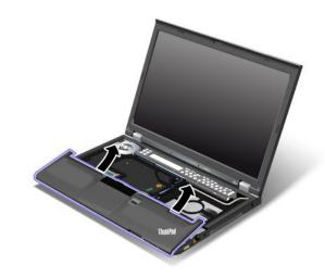
9. Release the palm rest from the computer. Now the palm rest has been removed.
