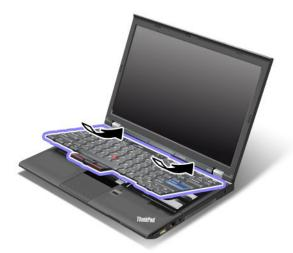
3. Press gently on the areas marked in the drawing, and slide the keyboard toward you. Make sure that the edges of the keyboard marked in the drawing, are under the frame.
