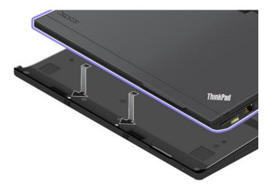
3. Make sure that the guides of the ThinkPad X220 UltraBase align with the holes of the computer 1. Then put the computer in place 2. The docking indicator lights.
