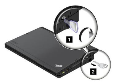
Note: You can turn the key clockwise to lock it. Then, keep the security key in a safe place. Do not lose this key; otherwise, you will be unable to detach the computer from the ThinkPad X220 UltraBase.
