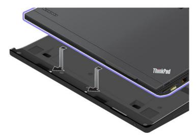
2. Make sure that the guides of the ThinkPad Battery 19+ align with the holes of the computer 1. Then put the computer in place 2.
