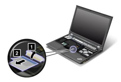
8. Lift up and remove the palm rest.
