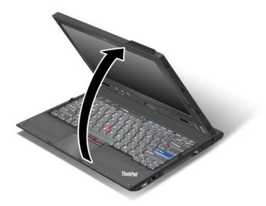
2. Open the display by at least 45 degrees, preferably by 90 degrees. Grasp the center of one side of the computer display with one hand while holding the keyboard bezel with the other hand; then rotate the display slowly clockwise until the back of the display is facing the keyboard. Your computer is now in the **picture frame mode**.
