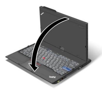
4. Press the center latch down to lock the display.
