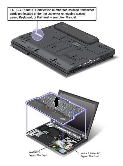
If no integrated wireless PCI Express Mini Card has been preinstalled in your computer, you can install one. To do this, follow the procedure in "Installing and replacing the PCI Express Mini Card for wireless LAN/WiMAX connection" on page 133 or "Installing and replacing the PCI Express Mini Card for wireless WAN connection" on page 139.
