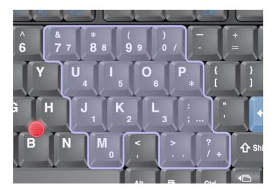
If the numeric keypad is enabled, press and hold **Shift** to use the cursor-control and screen-control keys temporarily.
