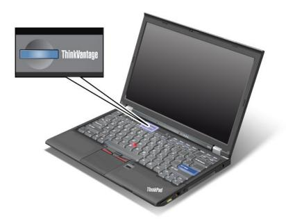
You can also use the ThinkVantage button to interrupt the startup sequence of your computer and start the Rescue and Recovery workspace, which runs independently of the Windows operating system and is hidden from it. If Windows is not running properly, you may need to do the following:
