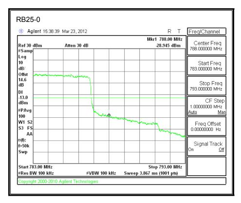
LTE 16QAM 784.5MHz Band 13, 783 - 793MHz (5MHz Bandwidth)
