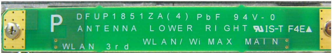
WLAN Main TX/RX Antenna
