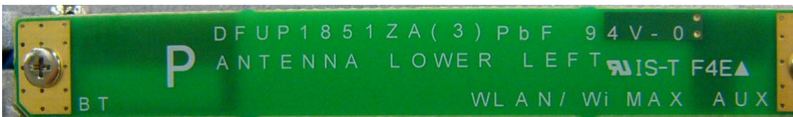
WLAN Aux TX/RX Antenna
