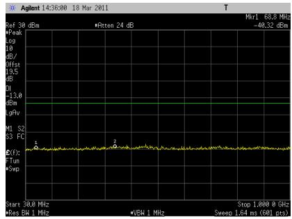
6.3.3.36 Out of Band Emissions at Antenna Terminals LTE B4, Low channel, 1715.0 MHz, 10MHz BW, 50RB, 16QAM, 1 GHz to 20 GHz
