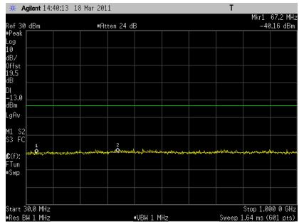
6.3.3.32 Out of Band Emissions at Antenna Terminals LTE B4, Mid channel, 1732.5 MHz, 10MHz BW, 50RB, QPSK, 1 GHz to 20 GHz
