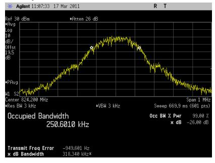
5.3.4.2 GMSK Occupied Bandwidth, Middle channel, 836.6 MHz, 99% bandwidth
