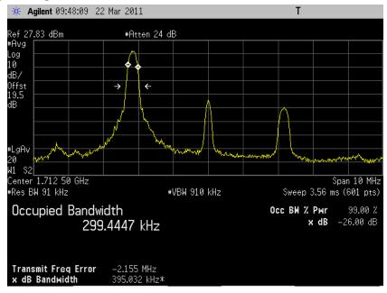
5.3.7.14 LTE Occupied Bandwidth, Band4 high channel (20375) BW=5MHz RB=1 RB Offset=24 QPSK 99% BW
