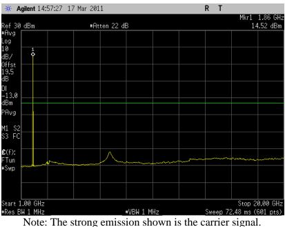
6.3.1.15 Out of Band Emissions at Antenna Terminals GMSK, Middle channel, 1880.0 MHz, 2 Hz to 1 GHz
