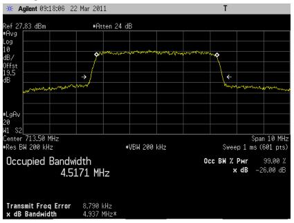
5.3.7.6 LTE Occupied Bandwidth, Band17 channel (23790) BW=10MHz RB=50 RB Offset=0 QPSK 99% BW
