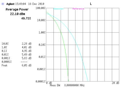
10.4.1.13 LTE peak to average ratio, 16QAM Band4, low channel, 1712.5 MHz, 5MHz BW, 25RB
