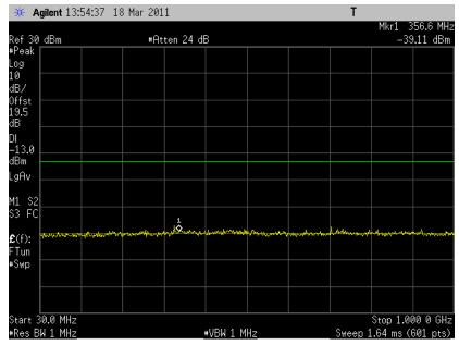
6.3.3.24 Out of Band Emissions at Antenna Terminals LTE B4, Low channel, 1712.5 MHz, 5MHz BW, 25RB, 16QAM, 1 GHz to 20 GHz
