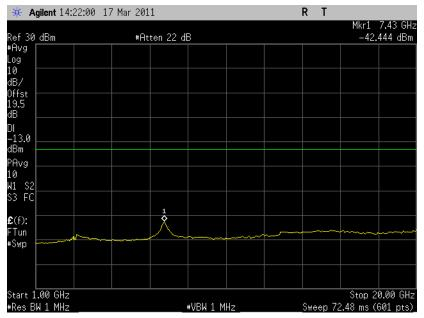
6.3.2.3 Out of Band Emissions at Antenna Terminals WCDMA, Middle channel, 836.4 MHz, 2 Hz to 1 GHz
