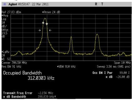
5.3.7.2 LTE Occupied Bandwidth, Band17 high channel (23825) BW=5MHz RB=1 RB Offset=24 QPSK 99% BW
