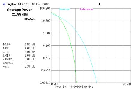
10.4.1.4 LTE peak to average ratio, QPSK Band17, high channel, 710 MHz, 10MHz BW, 50RB
