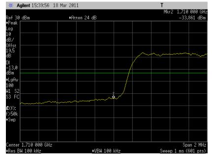
7.3.3.6 LTE; Band4 above 1755 MHz, with ch20375, 5MHz, QPSK, 25RB
