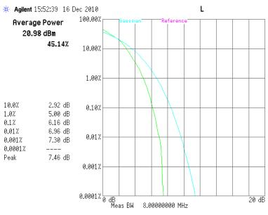
10.4.1.15 LTE peak to average ratio, 16QAM Band4, mid channel, 1732.5 MHz, 10MHz BW, 50RB
