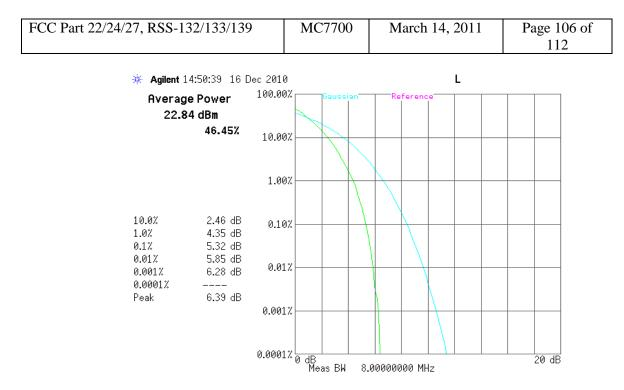
10.4.1.5 LTE peak to average ratio, 16-QAM Band17, Low channel, 706.5 MHz, 5MHz BW, 25RB
