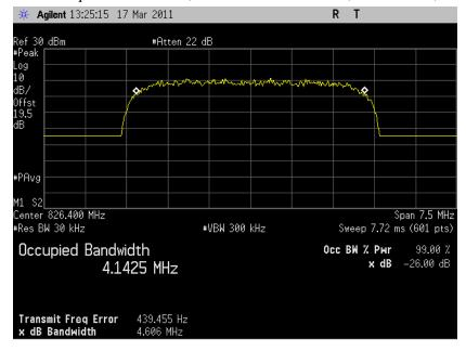
5.3.6.2 HSUPA Occupied Bandwidth, Cellular Middle channel, 836.4 MHz, 99% BW
