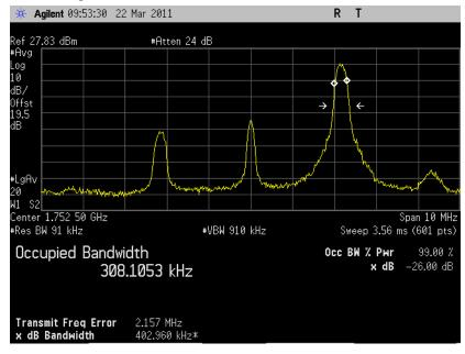
5.3.7.20 LTE Occupied Bandwidth, Band4 low channel (19975) BW=5MHz RB=25 RB Offset=0 16QAM 99% BW
