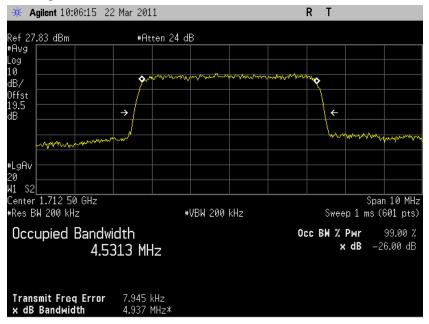
5.3.7.16 LTE Occupied Bandwidth, Band4 mid channel (20175) BW=5MHz RB=25 RB Offset=0 QPSK 99% BW
