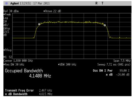
5.3.6.6 HSUPA Occupied Bandwidth, PCS High channel, 1907.6 MHz, 99% BW
