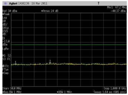
6.3.3.26 Out of Band Emissions at Antenna Terminals LTE B4, Mid channel, 1732.5 MHz, 5MHz BW, 25RB, 16QAM, 1 GHz to 20 GHz
