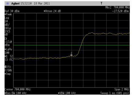
7.3.3.1 LTE; Band17 below 704 MHz with ch23755, 5MHz, QPSK, 25RB
