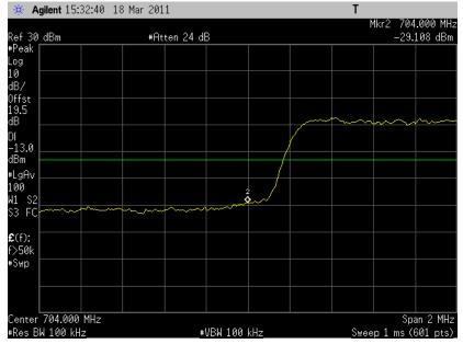
7.3.3.4 LTE; Band17 above 716 MHz, with ch23825, 5MHz, 16QAM, 25RB
