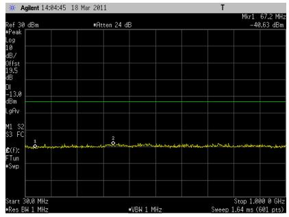
6.3.3.22 Out of Band Emissions at Antenna Terminals LTE B4, High channel, 1752.5 MHz, 5MHz BW, 25RB, QPSK, 1 GHz to 20 GHz
