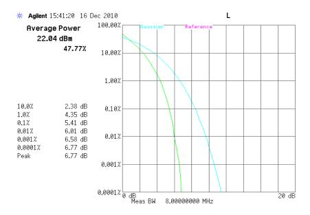
10.4.1.11 LTE peak to average ratio, QPSK Band4, mid channel, 1732.5 MHz, 10MHz BW, 50RB
