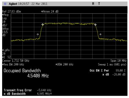
5.3.7.22 LTE Occupied Bandwidth, Band4 high channel (20375) BW=5MHz RB=25 RB Offset 16QAM 99% BW
