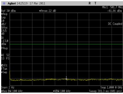
6.3.2.10 Out of Band Emissions at Antenna Terminals WCDMA, Middle channel, 1880 MHz, 1 GHz to 20 GHz
