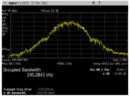
5.3.4.3 GMSK Occupied Bandwidth, High channel, 848.8 MHz, 99% bandwidth
