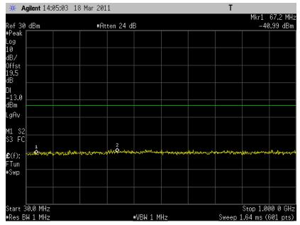
6.3.3.28 Out of Band Emissions at Antenna Terminals LTE B4, High channel, 1752.5 MHz, 5MHz BW, 25RB, 16QAM, 1 GHz to 20 GHz
