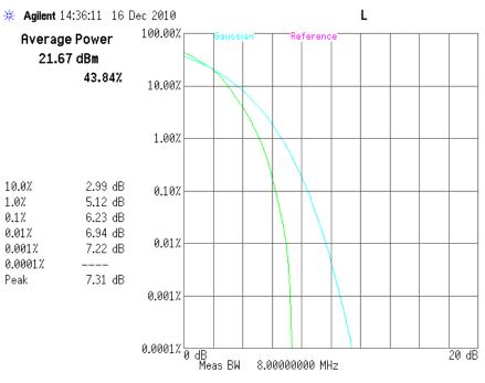
10.4.1.9 LTE peak to average ratio, QPSK Band4, low channel, 1712.5 MHz, 5MHz BW, 25RB
