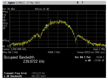
5.3.4.12 8-PSK Occupied Bandwidth, PCS High channel, 1909.8 MHz, 99% BW
