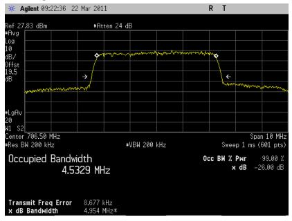
5.3.7.10 LTE Occupied Bandwidth, Band17 mid channel (23790) BW=5MHz RB=25 Offset=0 16QAM 99% BW
