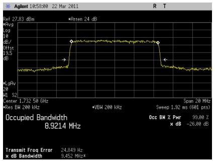
5.3.7.28 LTE Occupied Bandwidth, Band4 high channel (20734) BW=5MHz RB=25 16QAM 99% BW
