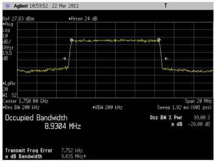
5.3.7.26 LTE Occupied Bandwidth, Band4 low channel (20000) BW=10MHz RB=50 RB Offset=0 16QAM 99% BW
