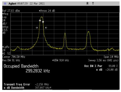
5.3.7.8 LTE Occupied Bandwidth, Band17 high channel (23825) BW=5MHz RB=1 Offset=24 16QAM 99% BW
