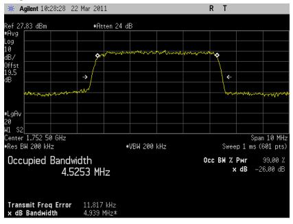
5.3.7.18 LTE Occupied Bandwidth, Band4 low channel (19975) BW=5MHz RB=1 RB Offset=0 16QAM 99% BW
