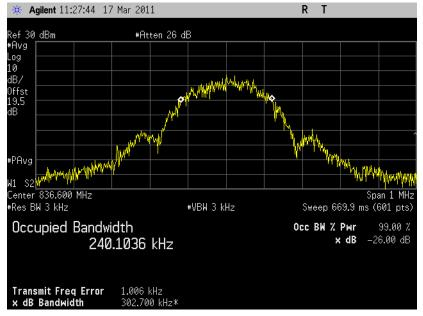
5.3.4.5 8-PSK Occupied Bandwidth, Middle channel, 836.6 MHz, 99% bandwidth
