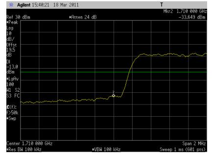
7.3.3.8 LTE; Band4 above 1755 MHz, with ch20375, 5MHz, 16QAM, 25RB
