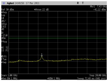
6.3.1.9 Out of Band Emissions at Antenna Terminals 8-PSK, Mid Channel, 836.6 MHz, 2 Hz to 1 GHz
