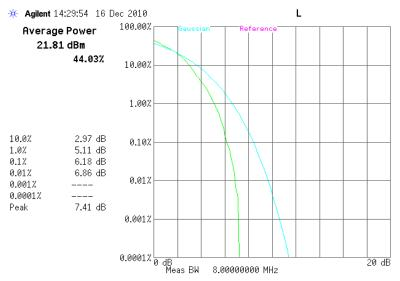
10.4.1.7 LTE peak to average ratio, 16-QAM Band17, Mid channel, 710 MHz, 10MHz BW, 50RB
