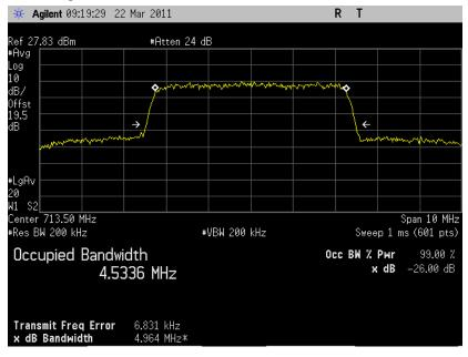
5.3.7.12 LTE Occupied Bandwidth, Band17 mid channel (23790) BW=10MHz RB=50 Offset=0 16QAM 99% BW
