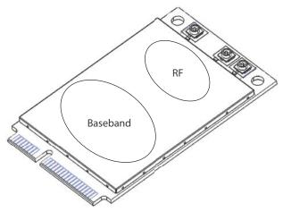
Figure 6-4: Shield locations (Top view)
