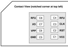
Figure 3-3: SIM Card Contacts (Contact View)
