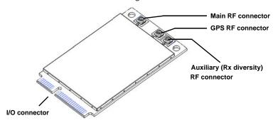
Figure 4-1: Module Connectors
