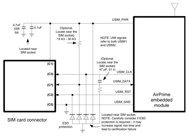
Figure 3-2: SIM Application Interface (applies to both SIM interfaces)
