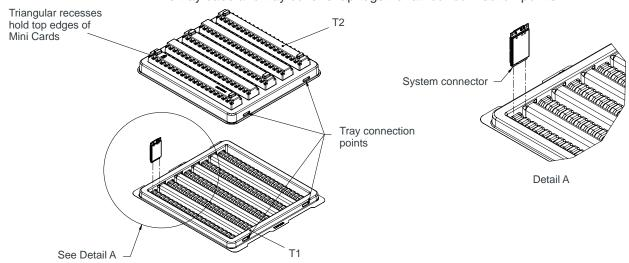
Figure 10-1: Device Placement in Module Tray
