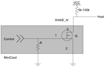
Figure 3-4: Recommended WAKE\_N Connection
