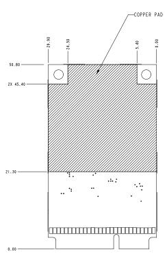
Figure 6-5: Copper Pad Location on Bottom Side of Module
