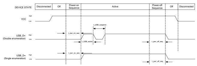
Figure 5-1: Signal Timing (USB Enumeration)
