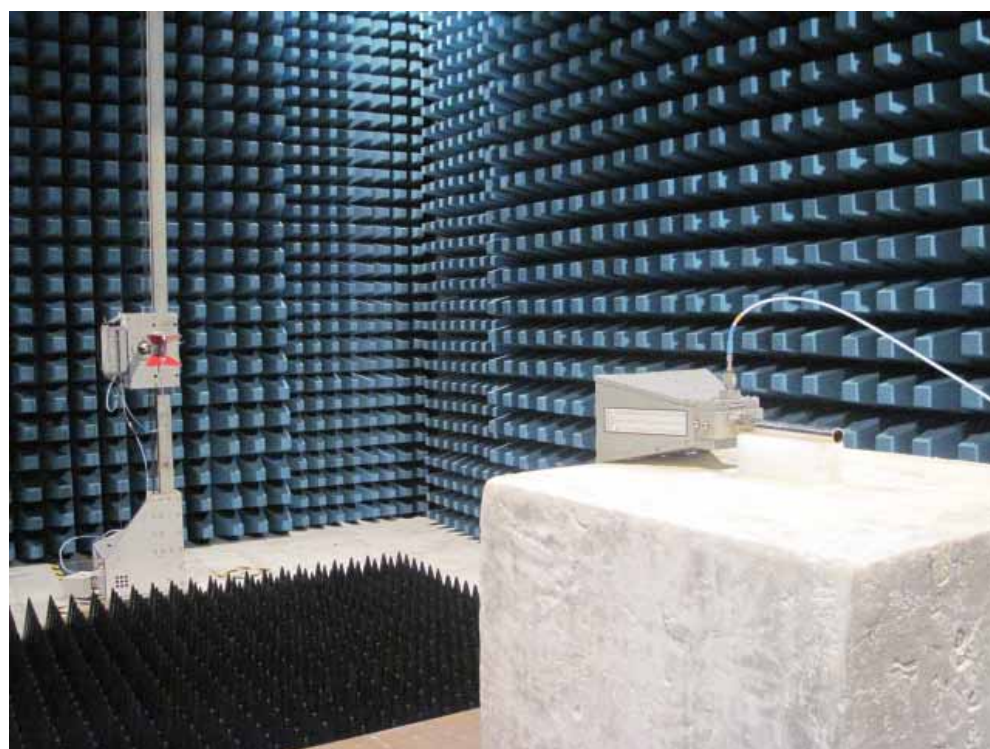
Description: Substitution Antenna for EIRP Test
