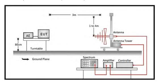
Radiated Spurious Measurement (above 1 GHz)
